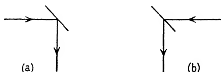
FIG. 14. Illustrating scattering at 90^\circ by a foil in the 'reflection' and 'transmission' cases (a) and (b) respectively.
